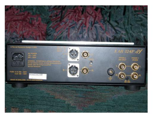
Rear view of the E.A.R. 324; inputs are to the right (Phono 1 for MC/MM is far right, while Phono 2 for MM only is one input set over), with the input selector button just under those RCAs. Ground is next over to the left. The two outputs are in the center.
