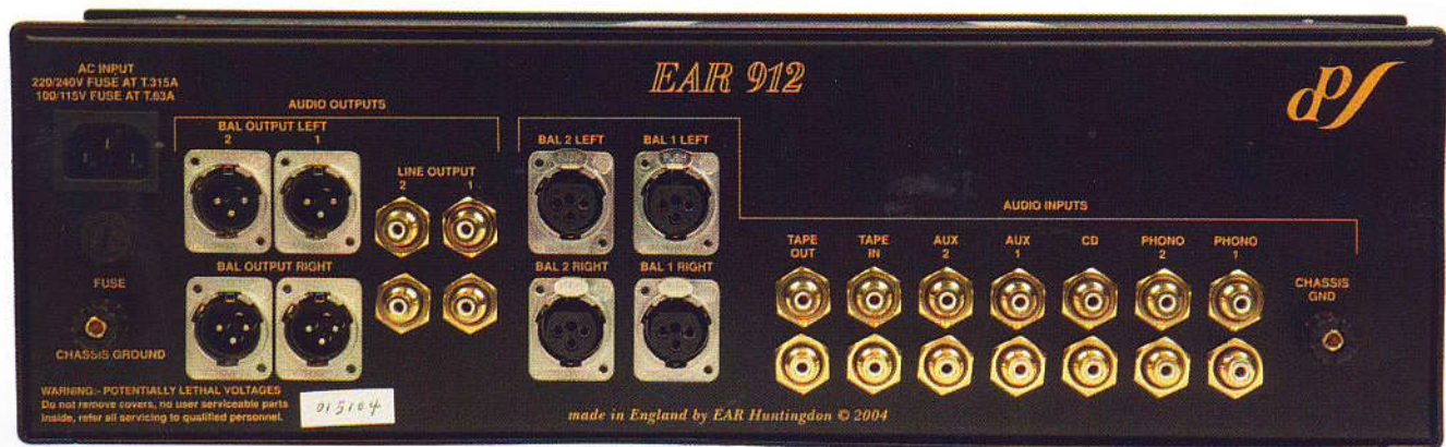
ABOVE: The back of the 912 features beefy connectors and two sets of balanced (XLR) and single-ended (RCA) outputs
